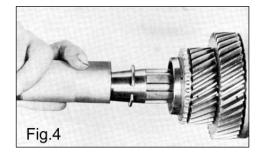
Those who own a lathe can make such cone themselves but I found that the Fig. 3 pliers, when used with some care do the job equally well. Since the circlip has to be put on the forward end of the splined shaft and is then pushed to its locking position, initial access is better so the risk of over-expanding the circlip is less than for the extracting procedure.
