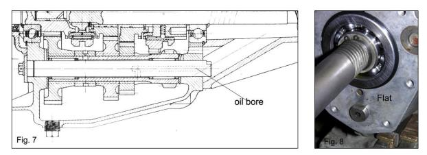
When fitting the front cover 71 with the lip seal 74 some care should be taken not to damage the seal by the splines. In the Service Instruction Manual it is recommended to use a seal guard as show in Fig. 9. The original lip seal is a leather seal and more prone to damage than the modern rubber lip seals. When taking care during
