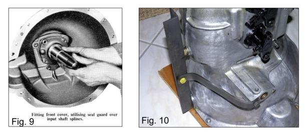
Manipulating the gearbox internals during assembly is much easier if the gearbox is stably held in a large vice. Fig. 10 shows an angle iron and strip and how these are fixed to the underside of the gearbox. The vice clamps on the angle iron. Fig. 11 shows the gearbox in its finished shape.
