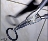
The advantage of this original tool is that the circlip is expanded on supporting fingers so that it might slide with little clearance over the splines and stress on the circlip is limited. As a consequence the circlip can, in principle, be reused. However, such a tool is no longer available (and I also think its price would be prohibitive...) and therefore an alternative had to be found for extracting the circlip.
