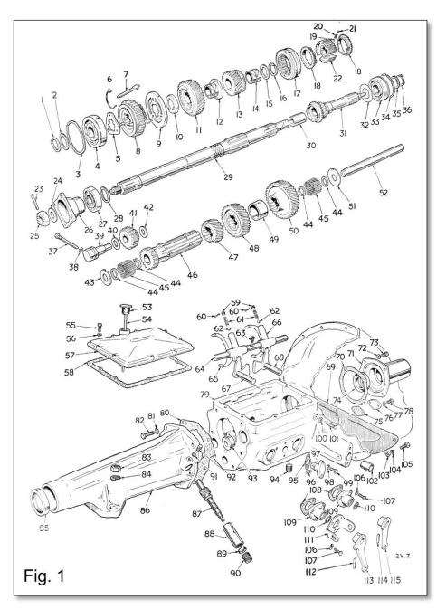
Disassembly is a straightforward job (the only difficulty I encountered was the removal of circlip 16 because initially I didn't have the right tool). The gearbox extension 86 and the bearings 4 and 33 could all be taken from the gearbox housing without the need of pullers. Some special tools are necessary and these tools or alternatives therefore will be described now.
