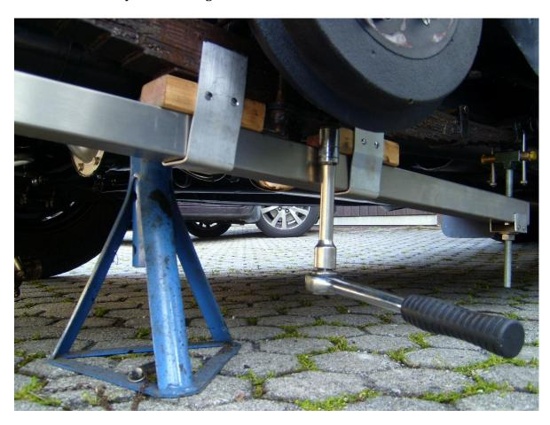
The supporting wooden blocks for contacting the middle of the spring are slidable and can so be adjusted to leave enough room for access to the nuts for the U-bolts.
