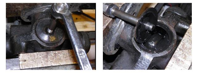
This success made me decide to use the same procedure for the metal disk opposing the damper arm rod end. It was found that the material of the disk is sufficiently thick to be able to cut a 1/8" BSP thread into a hole drilled at the center of the disk and by using the same threaded bolt the metal disk came out easily without any damage.
