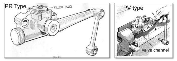
Both types have damper bore end-caps that can be unscrewed. In fact the PV6 can have either screwed-on or screwed-in caps or just core-plug end caps.
