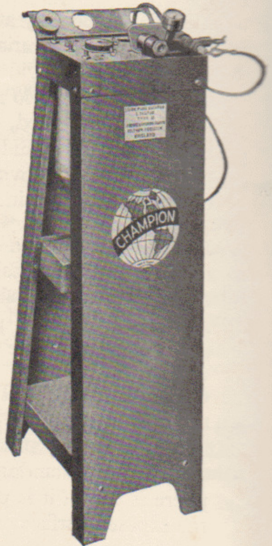
Fig. 32. Sparking plug cleaning and testing machine.
