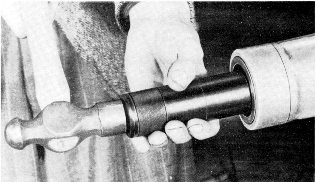
Fig. 36. Fitting ball-race in gearbox extension —Tool No. 20S-78.
